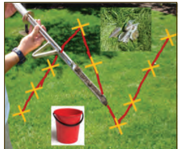
Fig. 2: Take 12 cores of soil by zigzagging to cover as much of the sampling area as possible.
